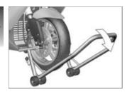
If the Scooter is raised too far at the front, the center stand lifts off the ground and the Scooter can tilt to the side. When raising the vehicle, make sure that the center stand remains on the ground. Adjust the height of the front wheel stand if necessary.
