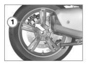
Check the brake pad thickness with visual inspection. Viewing direction: from lower right toward brake pads **1**.
