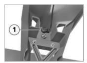
• Insert bulb socket **1** into lamp housing.
