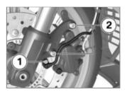
Install screws 2 on left and right with appropriate torque.
